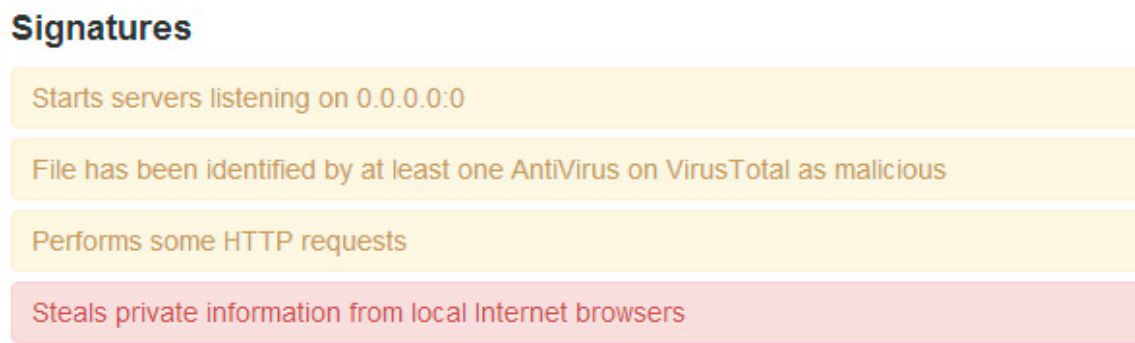
Figure 19. Signatures triggered by the Cuckoo on Static Analysis
